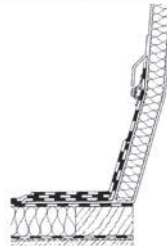
GRP RAK for SHEV with optional GFRP apron (protruding strips)
