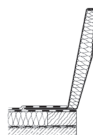
Steel aluminium composite upstand for SHEV RAK Model, 30 cm high
