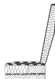
JET steel aluminium composite upstand for SHEV RAK Model, 30 cm high
