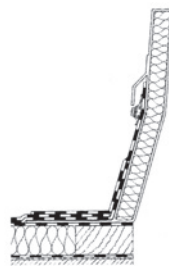
JET GRP RAK for SHEV with optional GFRP apron (protruding strips)
