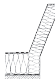
Steel aluminium composite upstand AK model 40 cm high
