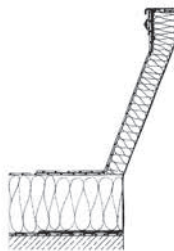
Metal upstand TE Model, 40 cm high with E-clamping rail
