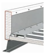
Continuous rooflight kerb for iso- and thermo roofs
